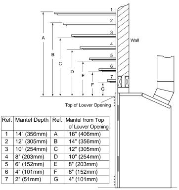
Figure 6 - Clearances for Combustible Mantels
